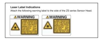
For details, including precautions for correct use, refer to the "ZS-HL Smart Sensor User's manual" (Cat. No. Z236) and "ZS-L Smart Sensor User's manual" (Cat. No. Z208) on your OMRON website.
